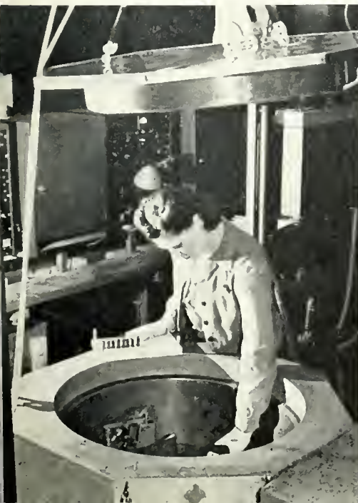
KATHERINE DANLEY LOADS AN AUTOMATIC DRUM TO GIVE THE FINAL TEST TO CRYSTAL BLANKS. THE DRUM REJECTS BAD CRYSTALS AUTOMATICALLY.
