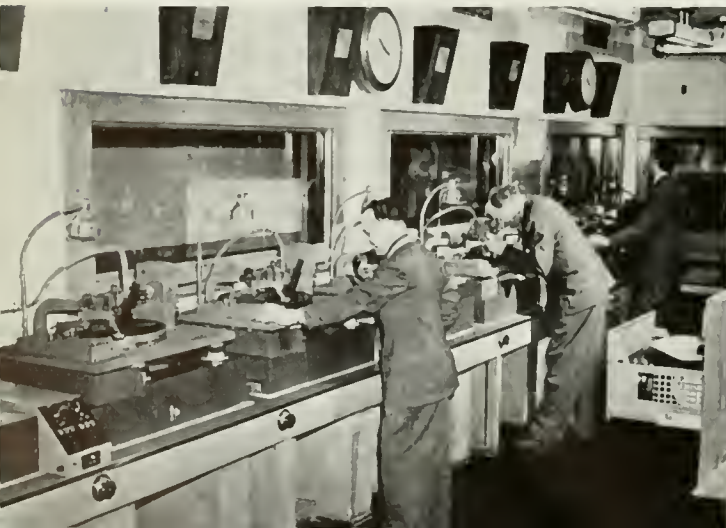
A SECTION OF THE RCA-BUILT RECORDING LATHE BANK AT OWI HEADQUARTERS IN NEW YORK CITY.
