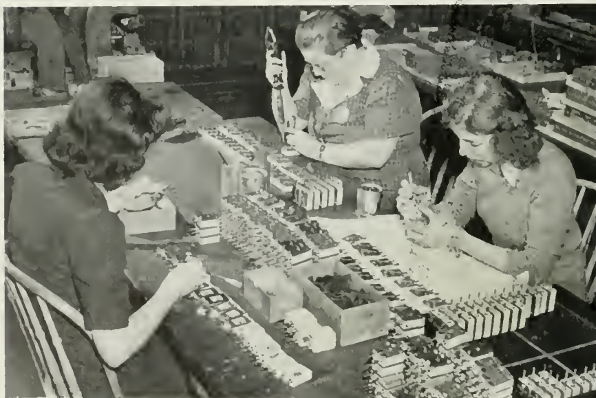
THESE GIRLS SOLDER AND ASSEMBLE CRYSTAL HOLDERS FOR USE IN RADIO AND ELECTRONIC EQUIPMENT FOR THE ARMED FORCES.
